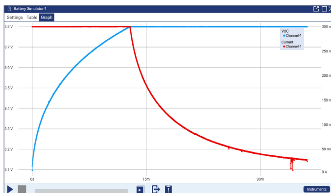
View VOC, Current, or ESR readings as they are collected during model generation.
